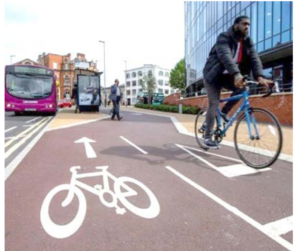
Figure 7.10 – Example of a floating bus stop in Leicester
