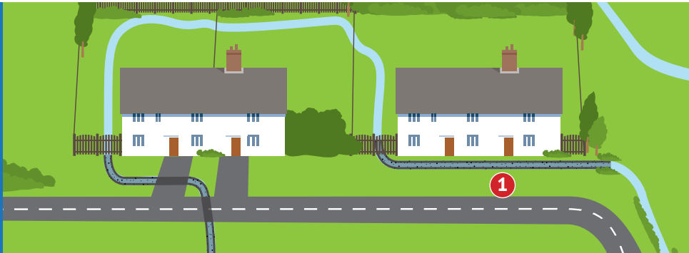
1 Culverted (piped) watercourse through land to the front of the property
