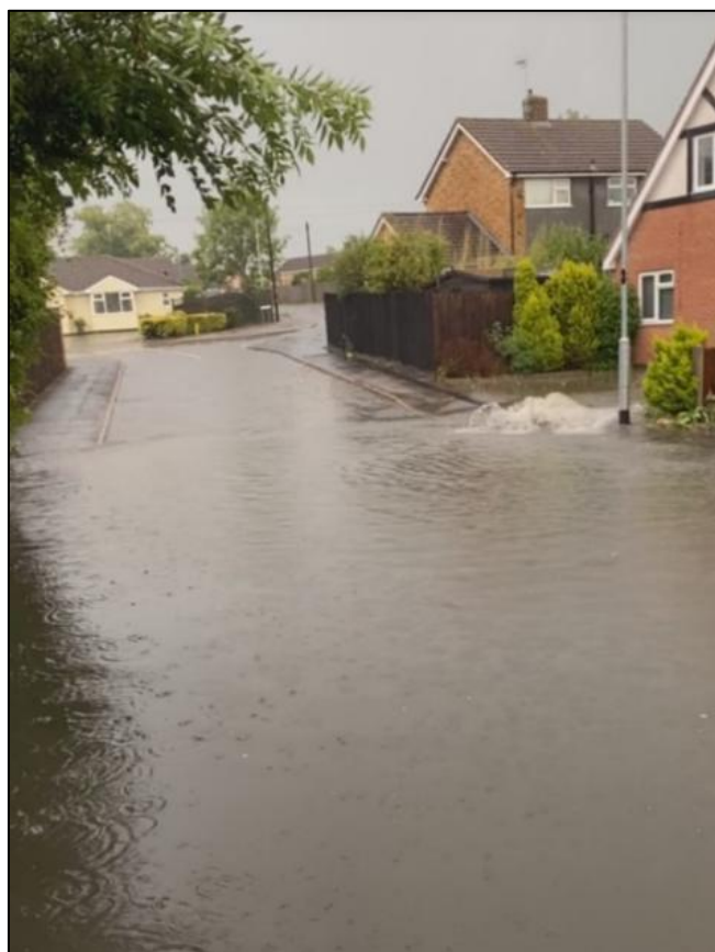
Photograph 19: Flooding and surcharged surface water network gully, Badgers Holt
