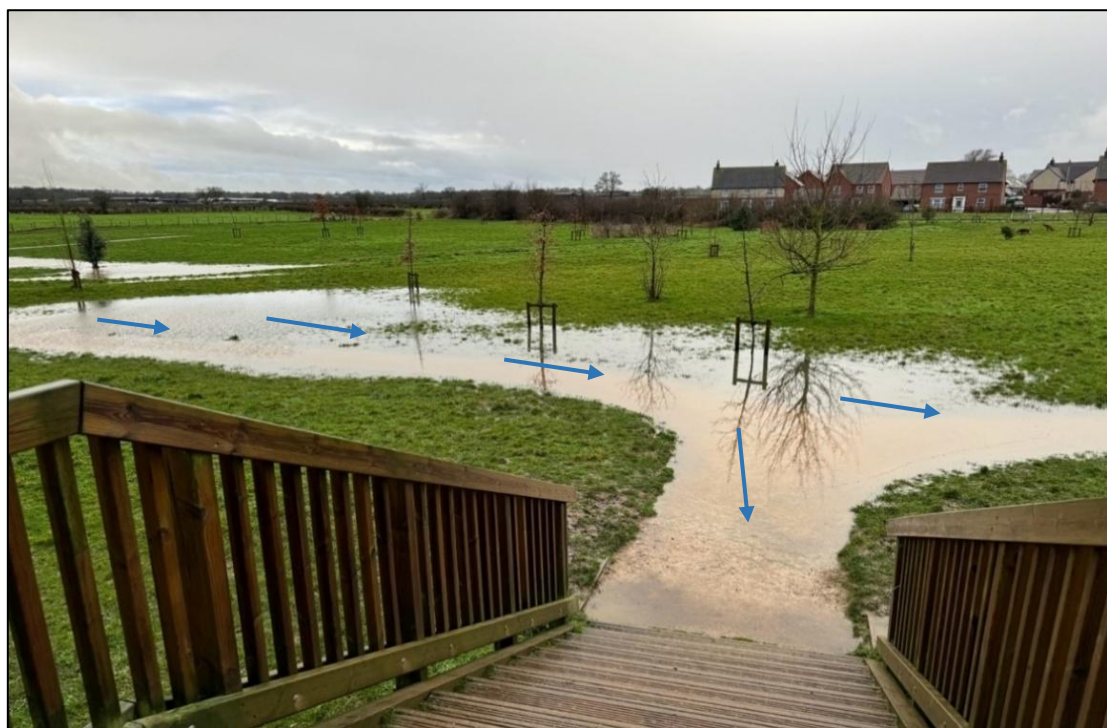
Photograph 11-3: Surface water flowing across public open space towards Elliott Close looking south towards Balancing Pond
