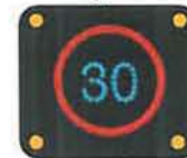
Proposed 30mph Vehicle Activated Sign with flashing amber lights
